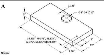
1. Center of electrical access is 7" from front & 2 1/2" from side of liner. Connection access is behind filters
