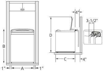
• To ensure sufficient clearance for water lines and airflow, allow minimum clearances of at least 1 in. (2.5 cm) at the sides and 4 in. (10 cm) behind the unit. Be sure to allow for wall, door, or floor moldings that may increase the required clearances.
