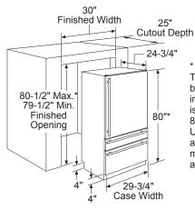
\* 80" High installation. The refrigerator can be adjusted to fit into a cutout that is 79-1/2" min. to 80-1/2" max. height. Use leveling legs and wheels for a maximum 1" height adjustment.
