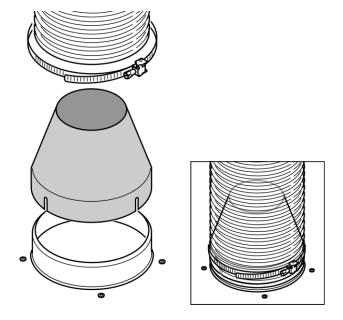
If you would like to reduce the environmental impact of your ventilation system by limiting the CFM output the Reducing Collar can be installed. It reduces the air flow to less than 300 CFM. Check local building codes for maximum CFM requirements.
