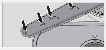
Spray arms can be removed for cleaning. Remember to fit them firmly back into place afterward.
