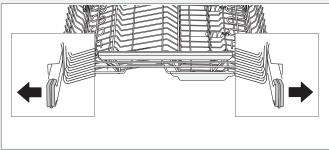
Remove the top cutlery tray. Push the top spray arm up and turn the spray arm bearings counterclockwise to remove the spray arm.
