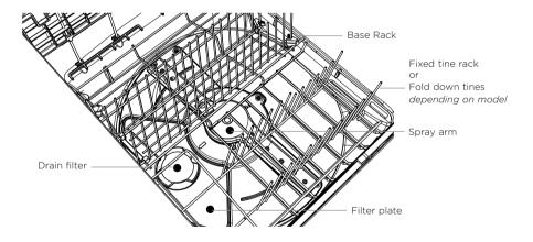
Cleaning the drain filter and filter plate
