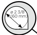
The ø 2 3/8" (60mm) services hole should be enlarged to accommodate the extra venting hose by cutting out some material from the bottom corner.
