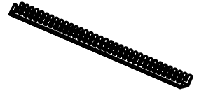
Edge Protector (1) (If the services hole is through a metal partition, the hole must be protected with the Edge Protector supplied to prevent damage to the power cord or hoses.)
