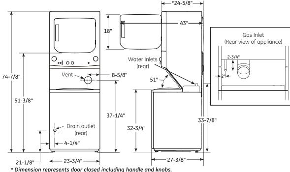
\* Dimension represents abor closed including handle and knobs NOTE: With feet set at mid position, feet can be adjusted +/- 3/8".
