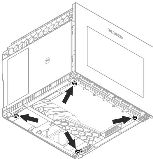
4. Adjust the feet to the required height if necessary. The feet can be turned by hand; if they do not turn easily, use the open-end wrench provided.
