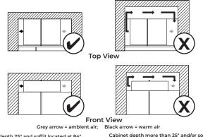
Cabinet depth 25" and soffit located at 84", provides proper airflow/ventilation to the refrigerator. Efficient cooling is achieved. Cabinet depth more than 25" and/or soffit located at more than 84", causes air gap at back and/or top of the refrigerator. Air gap allows warm air recirculation causing loss in cooling efficiency.
