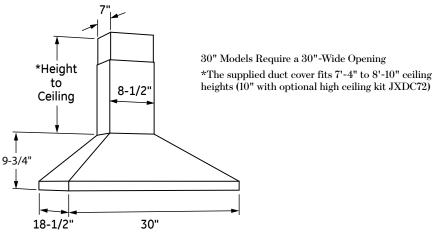
The vent hood must be installed 24" min. and 36" max. above the cooking surface. The hood installation height above the cooking surface depends upon ceiling height. The telescopic duct cover conceals the ductwork running from the top of the hood to the ceiling.
