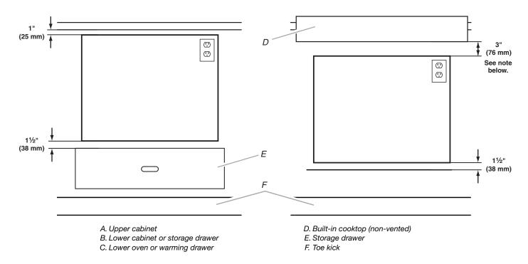
**NOTE:** The bottom of the cooktop may be sunk into the counter and lower cabinet. The minimum 3" (7.6 cm) clearance must exist below the lowest point of the cooktop, and there must be no interference between any part of the cooktop (including any gas fittings) and the microwave oven.
