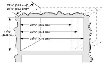
\*With flush receptacle, or with non-flush receptacle located in upper right or upper left corner of cutout.
