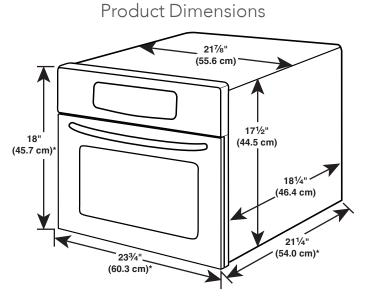
\*Measurements include front facing of microwave oven. Depth measurement also includes door handle.
