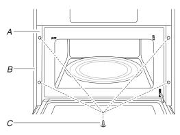
A. Microwave oven door facing frame B. Cabinet C. 1" T10 screws (4)
