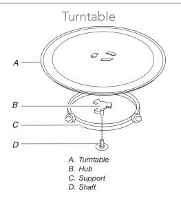
The turntable can rotate in either direction to help cook food more evenly. For best cooking results, do not operate the microwave oven without having the turntable in place. See the "Assistance or Service" section to reorder any of the parts.
