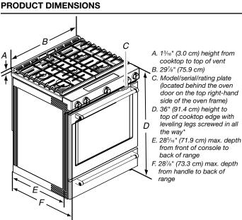
**IMPORTANT:** Range must be level after installation. Follow the instructions in the "Level Range" section. Using the cooktop as a reference for leveling the range is not recommended.
