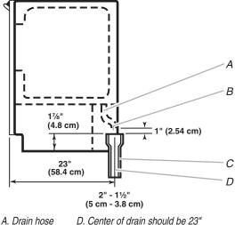
B. 1" (2.54 cm) air gap C. PVC drain reducer D. Center of drain should be 23" (58.4 cm) from front of door, with or without the ¾" (1.91 cm) panel on the door. The drain should also be centered from left to right (75%e" [18.56 cm] from either side of the ice maker).
