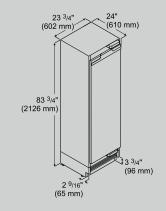
IMPORTANT! Stated minimum height dimensions include when the leveled feet are fully inserted.
