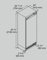
Stated minimum height dimensions include when the leveled feet are fully inserted.
