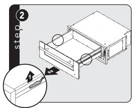
Slide finger along right and left side until you reach the hand latches (located approximately in the center of the rail). Pull up on on the left side latch and press down on the right latch at the same time and pull out the drawer pan.
