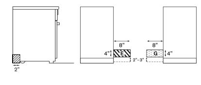
Installation clearance available behind range Electrical Installation Location Gas Installation
