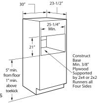
• Oven overlaps will conceal cut edges on all sides of the opening. **Note:** PSB9120 series Advantium can be installed below GE/GE Profile non-downdraft gas and electric cooktops. It CANNOT be installed below induction or Monogram (2GU3841385) gas cooktops.
