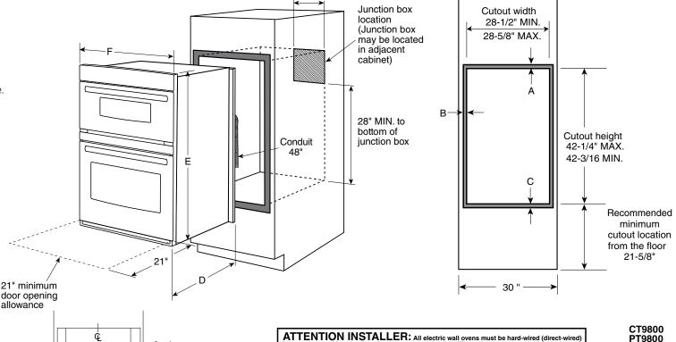
NOTE: If the cabinet does not have a solid bottom, two braces or runners must be installed to support the weight of the oven. For single ovens, the runners and braces must support 200 lbs (91 kg). For double ovens, the runners and braces must support 375 lbs. (170 kg).
