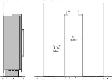
(a) Area to be left clear for the anti-tipping brackets -3"1/2x5" (82x127mm)
