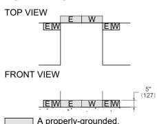
A properly-grounded, horizontally-mounted electrical receptacle should be installed according to this drawing.
