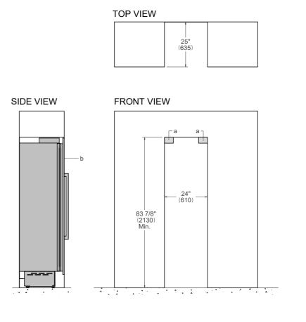
(a) Area to be left clear for the anti-tipping brackets – 3"1/2x5" (82x127mm)
