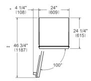
\* Maximum Overall Handle Dimension \*\* Width of 3/4" (19mm) Door Panel
