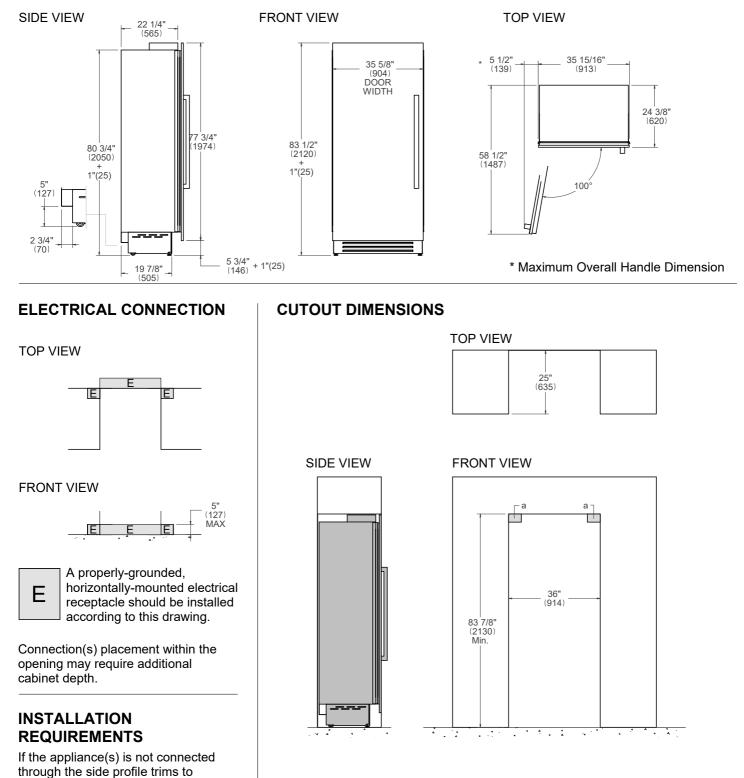
(a) Area to be left clear for the anti-tipping brackets  $-3^{\circ}1/2x5^{\circ}$  (82x127mm)
