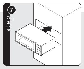
Slide cavity assembly into the cabinet opening.
