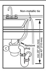
Note: Plumbing installations will vary - refer to local codes. Drain hose included is 88 5/8" (225 cm) and can be extended to a maximum of 165 3/8" (420 cm).
