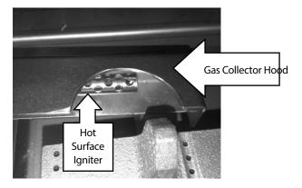
If the burner will light with a match, then the igniter may not be functioning correctly. Call for service.
