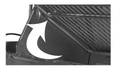
Then mount the skewer on the grill before lighting the rotisserie infrared burner. Lighting the burner first could result in burning your hands while trying to mount the skewer on the grill.
