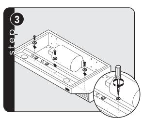
Attach with screws and lock washers provided.
