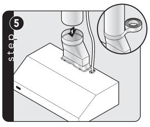
Slide duct over transition and tape around joint.
