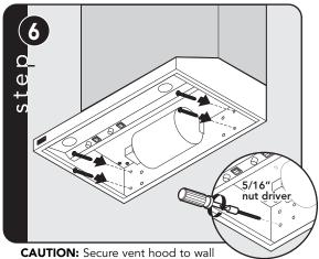
using screws provided. Use additional mounting screws and wall anchors, if necessary.
