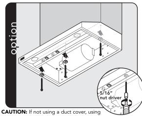
screws provided, make sure top mounting screws are secured into soffit or cabinet framing. Use additional mounting screws, if necessary.
