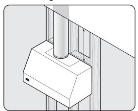
**NOTE:** Because of the weight of the hood make sure that the mounting screws are driven into the framing and not just the drywall. It may be necessary to drill additional holes in the canopy for proper alignment.
