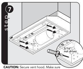
mounting screws are secured into framing. Use additional mounting screws and wall anchors, if necessary.
