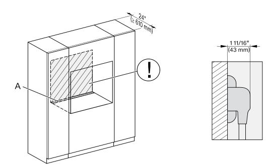
A - Cut-out (4" x 28" [100 mm x 720 mm]) in the bottom of the cabinet for the power cord and Ventilation
